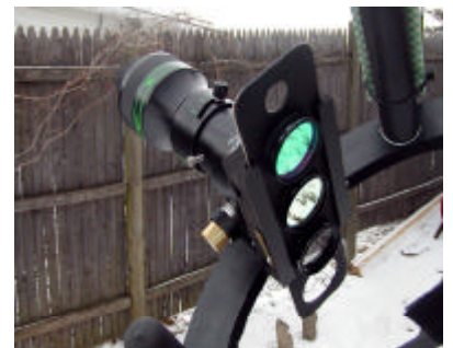
A filter slide provides safe and easy access to your filters. Photo used with permission. www.Astrocrumb.com
